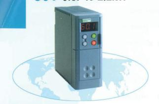
The 601 series inverters are designed for highly cost effective speed control of standard three phase induction motors from either single phase (nominal 230V) or three phase (nominal 400V) ac supplies. Ratings are available from 0.37 to 2.2kW and each unit is compatible with the Smart Card programming facility that provides simple copying or storage of drive set-up data.
