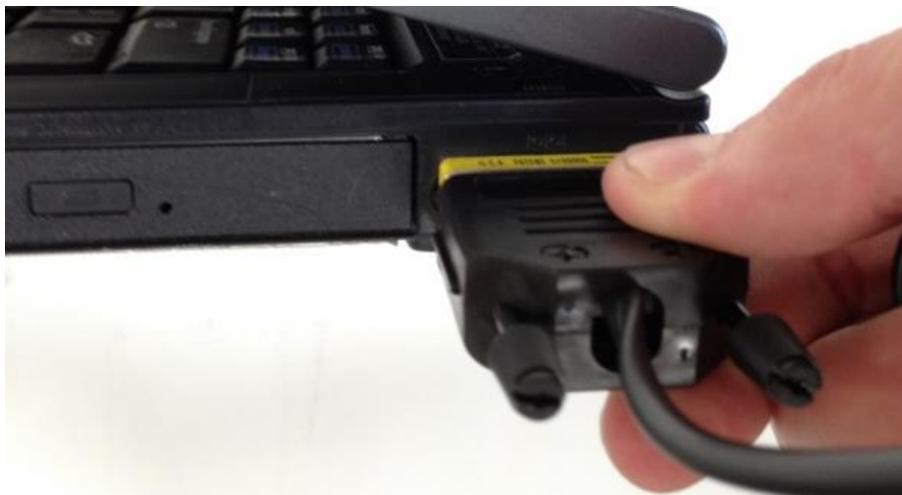
If your computer or laptop PC **does not** have a serial port, you will need to **USB to SERIAL PORT Adapter**. As seen below;
