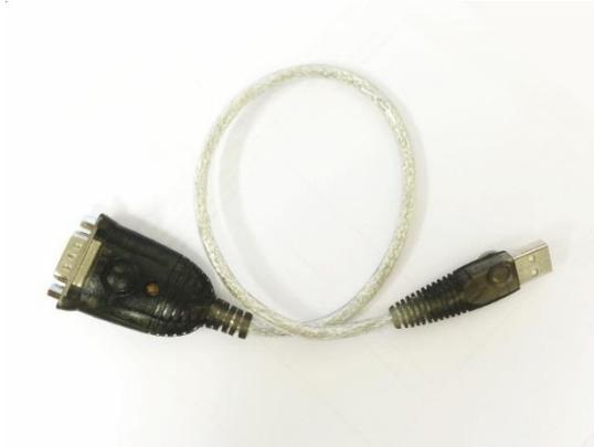
Connect the male and female ends of the serial adapter and your LA387599 comms lead.
