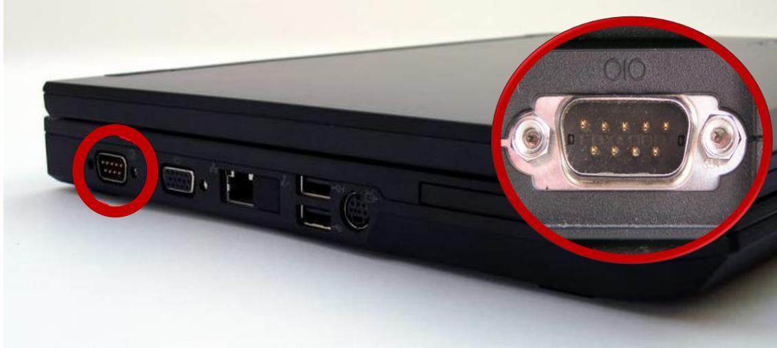
If you're computer or laptop PC **does** have a serial port, plug your LA387599 PC to Drive comms lead into this port as seen below;
