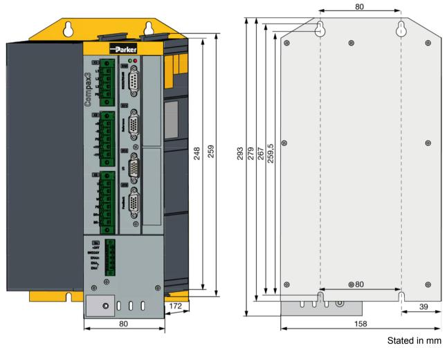
Please respect an appropriate mounting gap in order to ensure sufficient convection:
